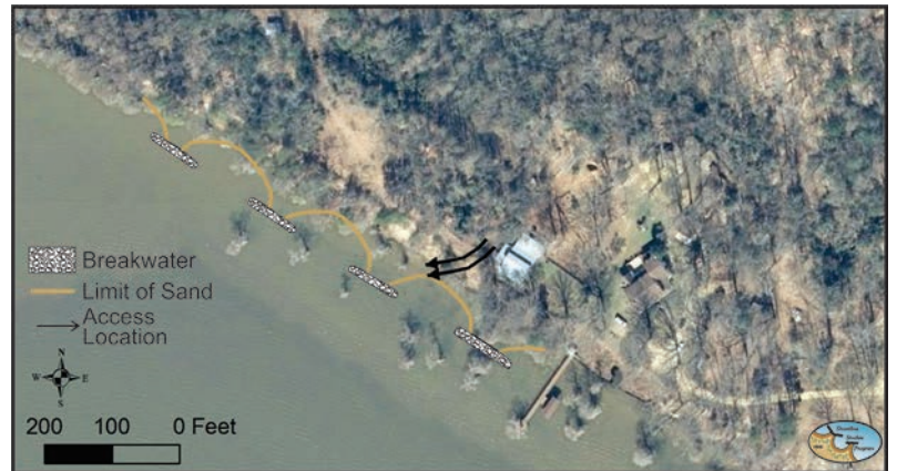
Figure 5-7. Proposed configuration of Shoreline BMP for Sturgeon Point.
