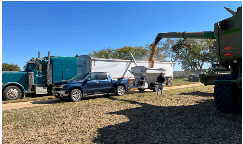
District staff use a weigh wagon (mobile scale) to measure the volume of soybeans harvested, which will then be used to calibrate the combine's electronic yield monitoring system.
